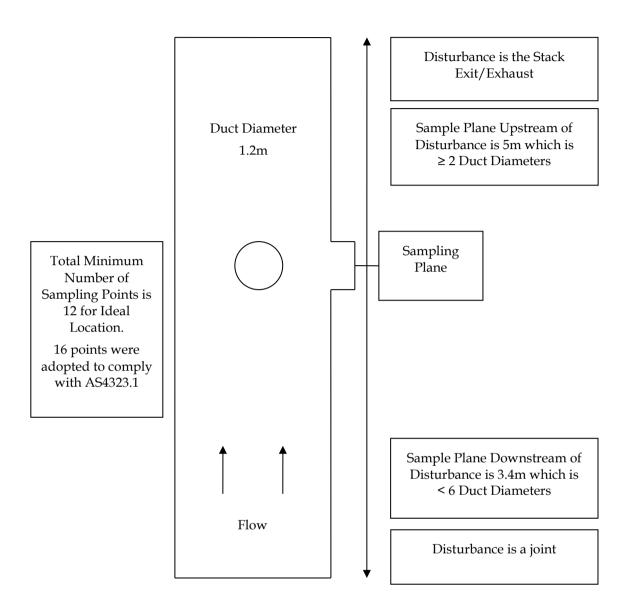
In the absence of cyclonic flow activity ideal sampling plane conditions will be found to exist at 6-8 duct diameters downstream and 2-3 duct diameters upstream from a flow disturbance. The sampling plane does not meet this criterion. Additional sample points were used in compliance with AS4323.1 as the sampling plane was non-ideal.
