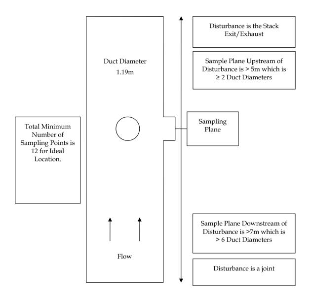
FIGURE 1-2 EPA NO.2 SCRUBBER STACK SERVING THE HOT BLOCK STORE
